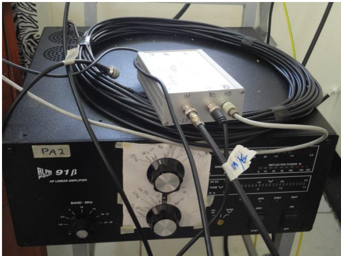
1.5kW amp and filters for beves
